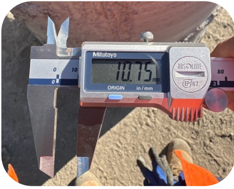
Hardfacing measurements before and after 5570mm of drilling – With Complex42™
