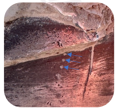
Reference location marks in barrel for measuring the height of the hardfacing
